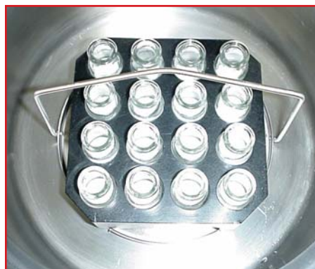
Shelf handle allows lowering the shelf onto the condenser surface for rapid vial freezing
