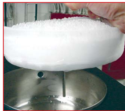
Shelf can also serve to rapidly remove the collected ice when defrosting
