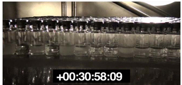
Figure 7. Photo of uncontrolled nucleation in a freeze dryer. 7
