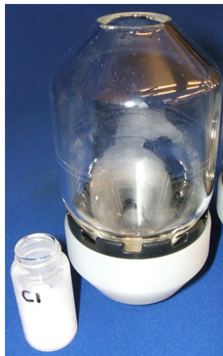
Figure 6 – Flask showing minimal sample sticking with added 1,4-dioxane
