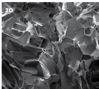
**Fig 2.** Effects of controlled nucleation using ControlLy. A) Freezing temperatures of products during uncontrolled nucleation vary considerably, B) consistent freezing temperature of drug products during controlled nucleation with ControlLy, C) small, irregular crystals of sucrose (75 mg/mL) during uncontrolled nucleation using 10C/min shelf cooling rate, D) larger, more consistent crystals of sucrose (75 mg/mL) during controlled nucleation with ControlLy at -30C shelf cooling rate.
