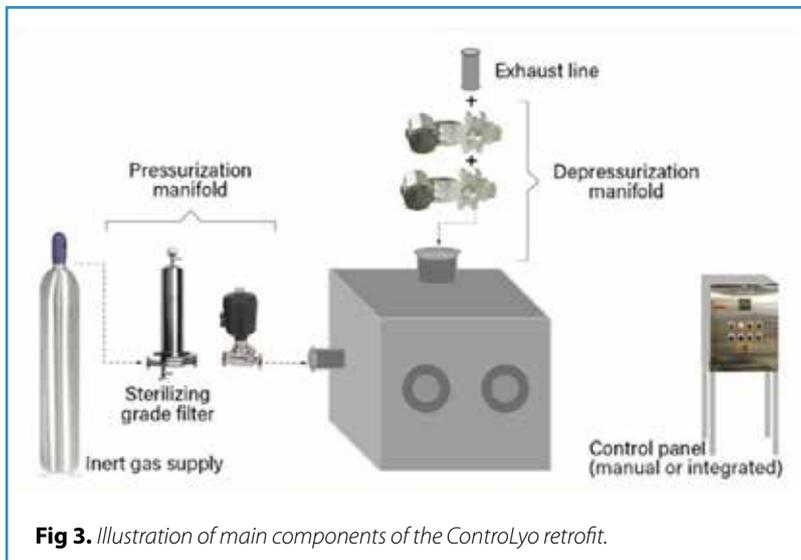
**Fig 3.** Illustration of main components of the ControlLyo retrofit.
