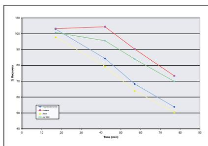
Figure 3. Stability of pesticides in toluene under vacuum
