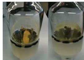
Figure 1. Benzanthrone remaining in the SampleGenie after 1st drying step (left) and 2nd drying step (right)
