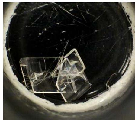
**Photo B:** Adipic Acid & Carbamazepine co-crystallised from ethanol
