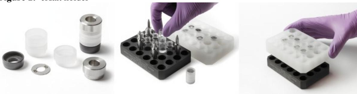
L to R: eXalt baffles and tower assembly, loading vials and towers to holders, completed holder assembly
